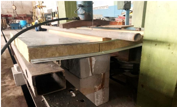
Fig. 1. Layering of the insulation on the support to a width of up to 4.5 mm after applying the maximum load
